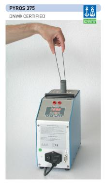
It covers a range from 10 °C above ambient temperature up to 375 °C. It has a stability of  $\pm 0,15$  °C and an accuracy of  $\pm 0,25$  °C at 150 °C. of  $\pm 0.35$  °C at 375 °C.
