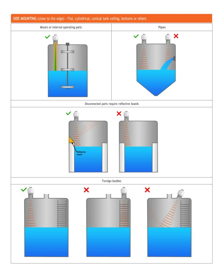
To calculate the minimum distance to the edge of the tank:
