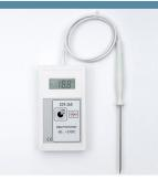
DT-34 is made of ABS material which protects the device from mechanical damage. Due to a hermetic construction of the device, it is resistant to dust, dirt and moisture.
