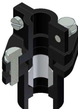
teflon sealing ( up to +200°C )
