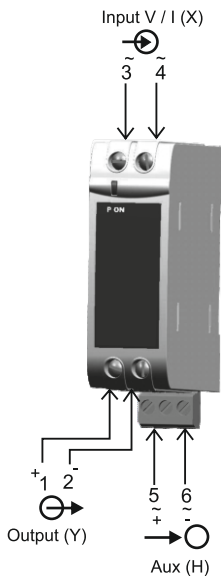
Fig. 6. Front View of Device for electrical Connections
