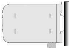
Fig. 3 Top-hat rail Mounting
