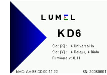
Fig.7 The recorder screen after turning on the power
