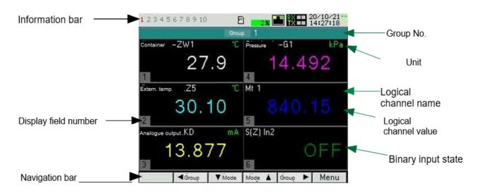
Fig.8 KD 6 recorder front panel
