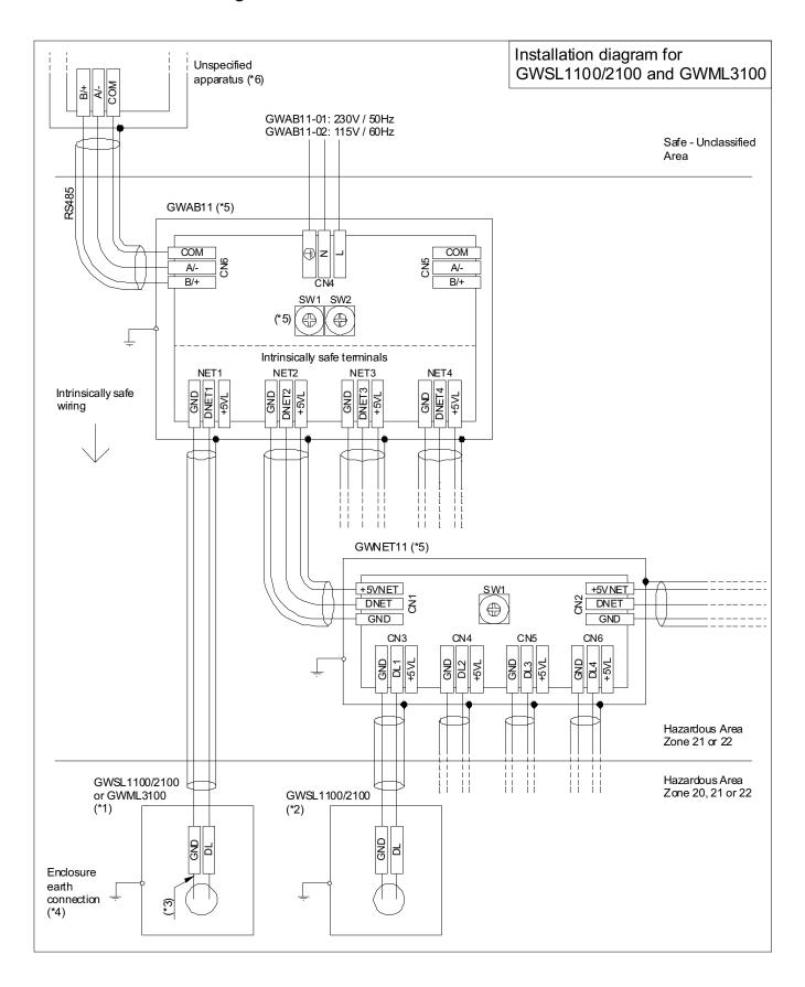
The installation diagram shows a typical installation using a GWAB11 as the intrinsically safe associated apparatus, i.e. the barrier and a GWNET11 to extend the number of sensor cable inputs in the GWAB11.
