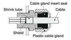
The shield, at any end of the cable, MUST NEVER, under any circumstance, be connected to GND or any other terminal in the sensor cables, the GWNET11 or the GWAB11/12.
