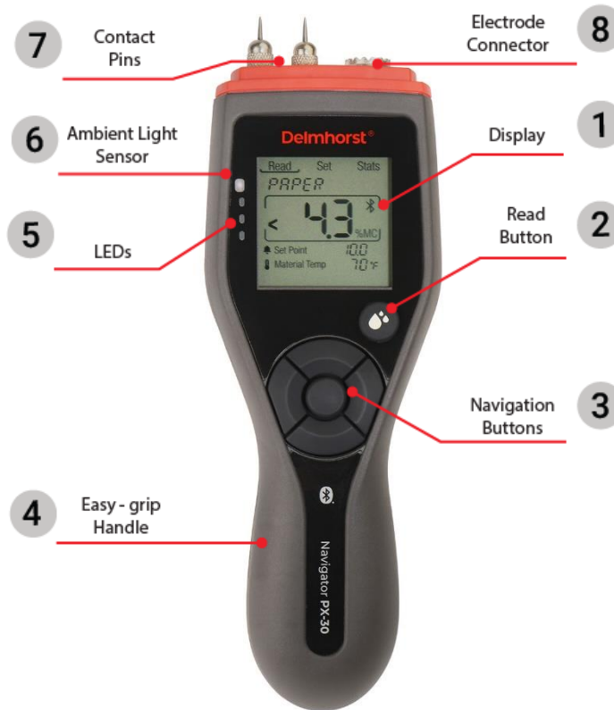
Figure 1: Meter components
