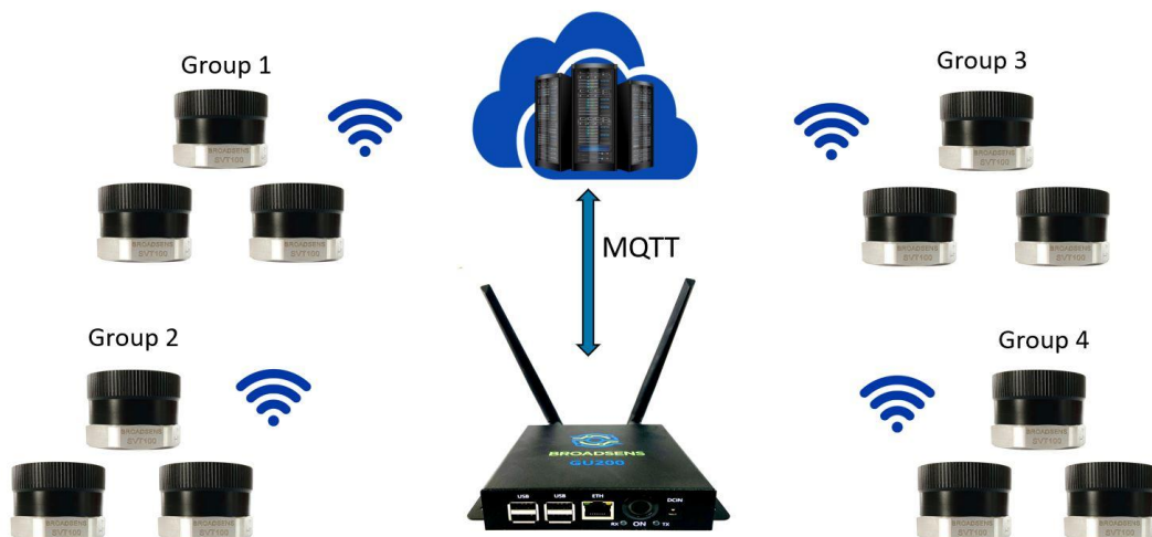
Figure 1 Group control of multiple wireless sensors
