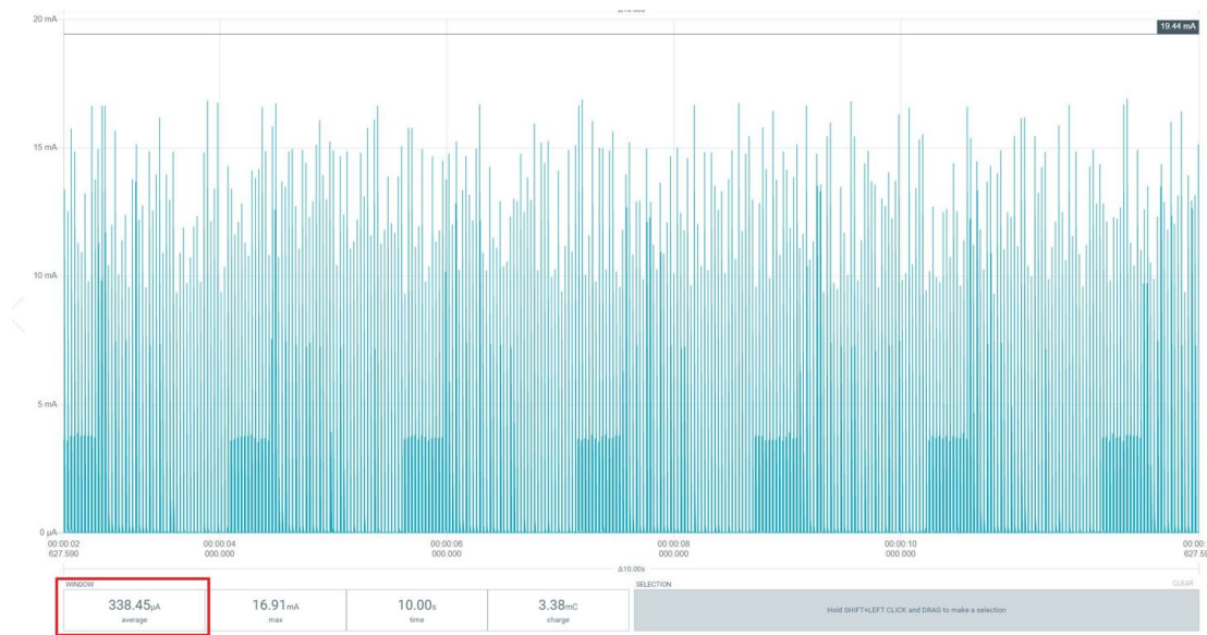
Figure 33 Single DAQ mode power consumption after DAQ, only transmission
