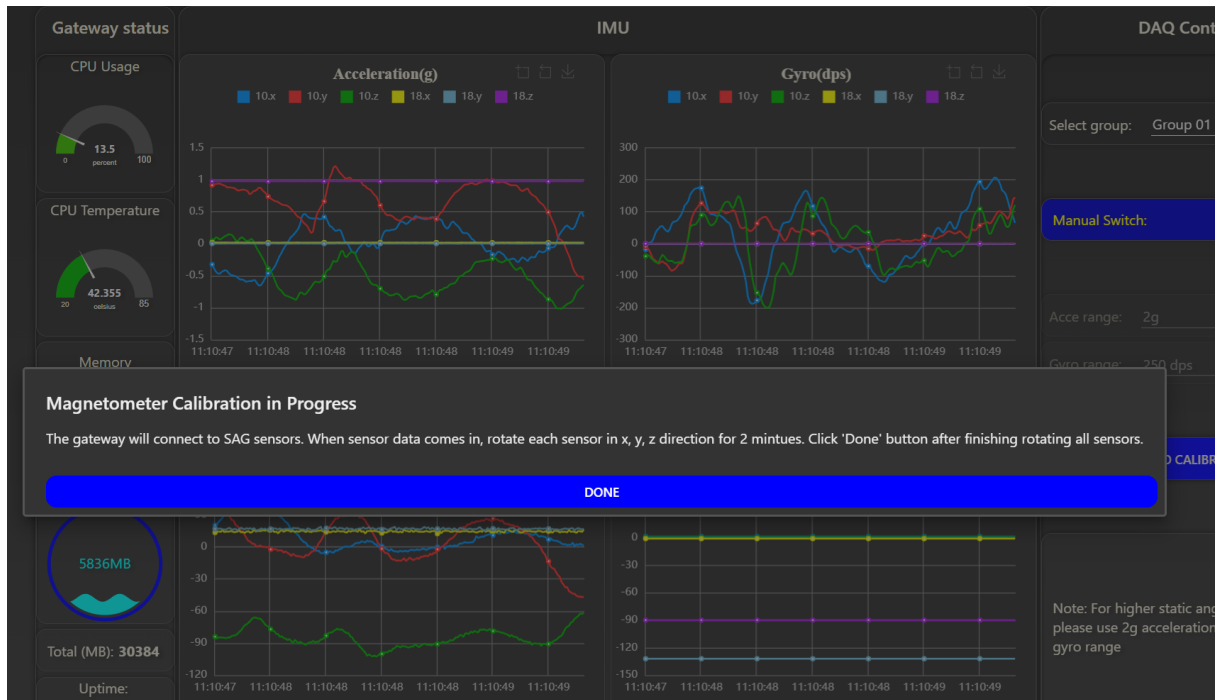
Figure 107 Magnetometer calibration in progress
