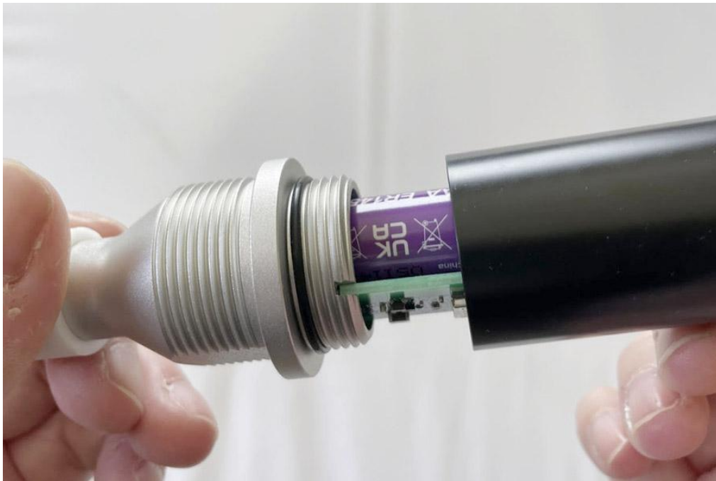
Figure 112 Unscrew sensor cover
