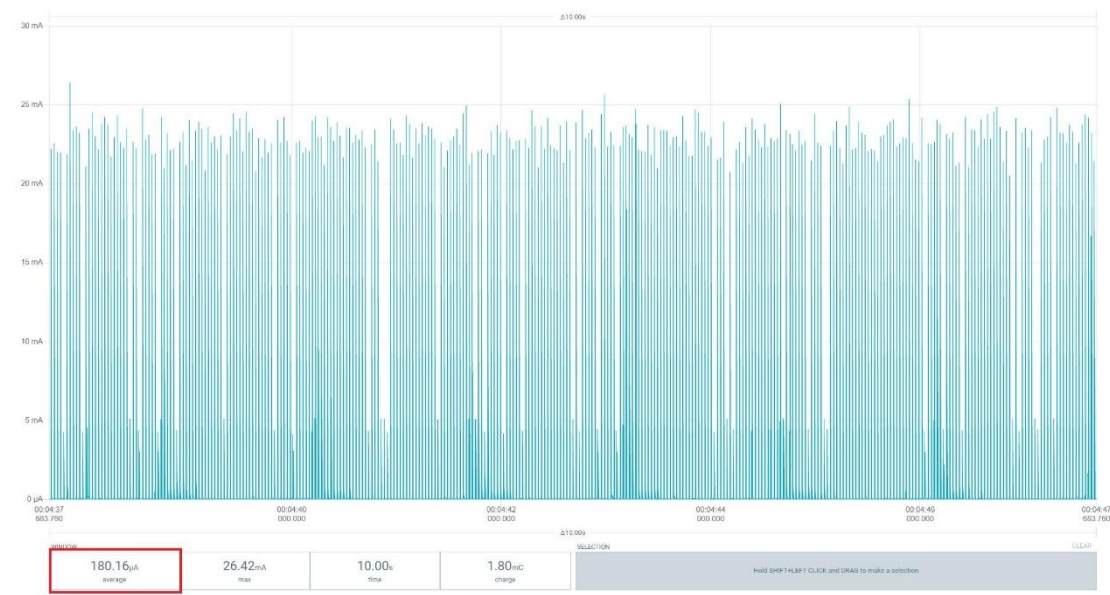
Figure 26 Power consumption of SVT-A series sensor in real-time mode 50Hz
