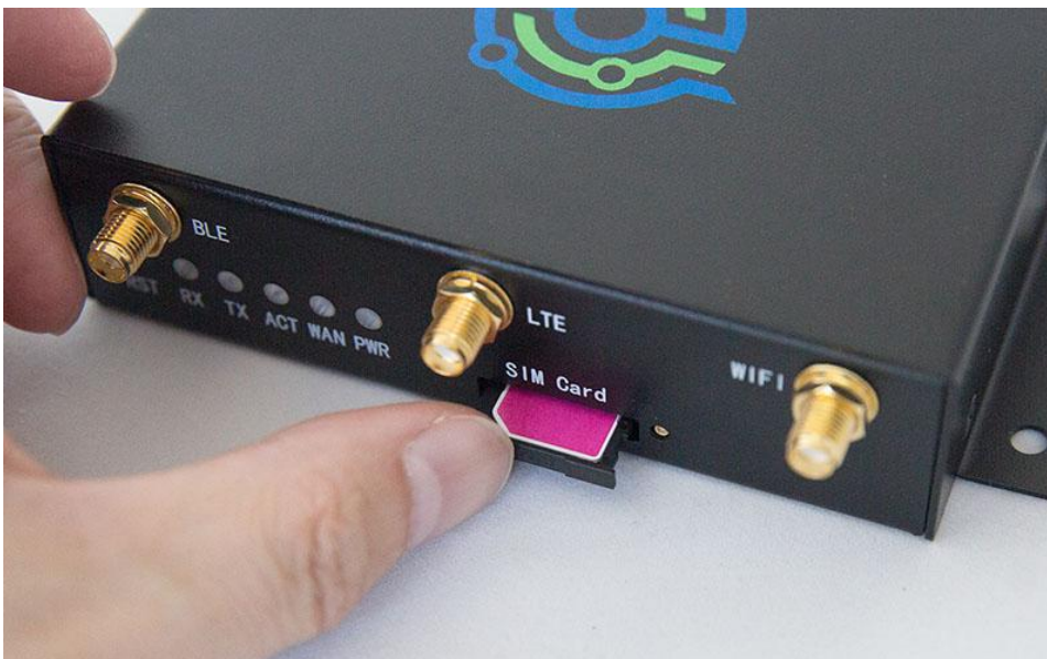
Figure 11 Insert SIM card tray to GU300S
