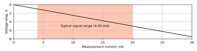
Please consult the documentation of the external  $4-20\,\text{mA}$  signal source to verify that a load of  $250\,\Omega$  and the associated voltage drop are applicable to the particular device. Failure to observe these constraints might result in unstable operation or damage to the  $4-20\,\text{mA}$  signal source device.
